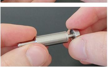
Step 11: Place the front bearing on the shaft.
