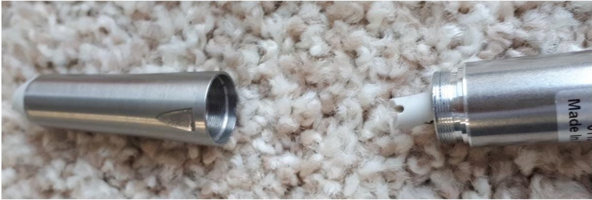
If necessary, unscrew the motor from the inner core of the hand piece.
