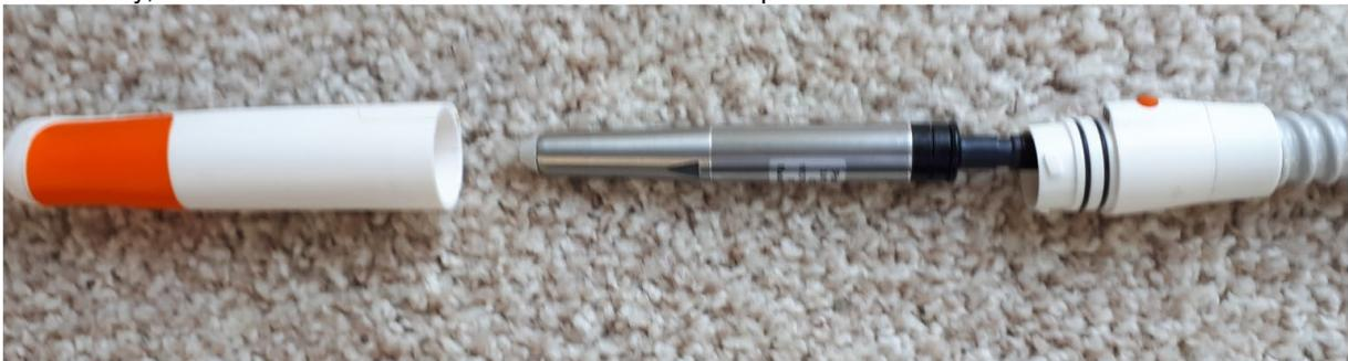
When reassembling, insert the inner core with motor into the front section of the hand piece casing.
